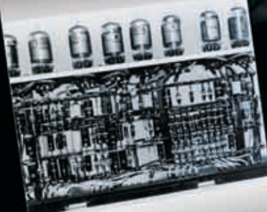
~ 1951 Vacuum Tubes Electronic devices with glass/steel vacuum envelope and electrodes. The first commercial usage of this technology was Univac, IBM 701.
